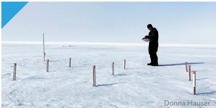
**On ice measurements** Responding to recent sea ice thinning, Ikaagvik Sikukun measures sea ice growth and melt over the winter and spring, and tracks snow depth, which insulates the ice keeping it warmer in winter (less sea ice growth) and cooler in spring (less ice melt).
