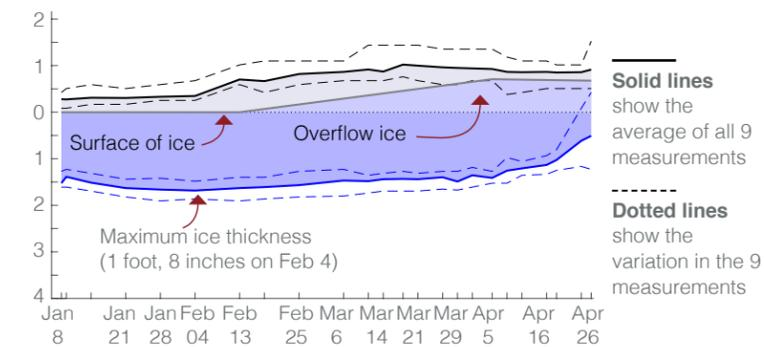
**2019 bay site** Bay site ice stopped growing three months earlier than usual and was over a foot thinner than 2018. Strong southerly winds and deep February snow pushed the surface of the ice down, causing overflow. By winter's end overflow was ~1 foot 5 inches thick, making up 50% of the total ice thickness.
