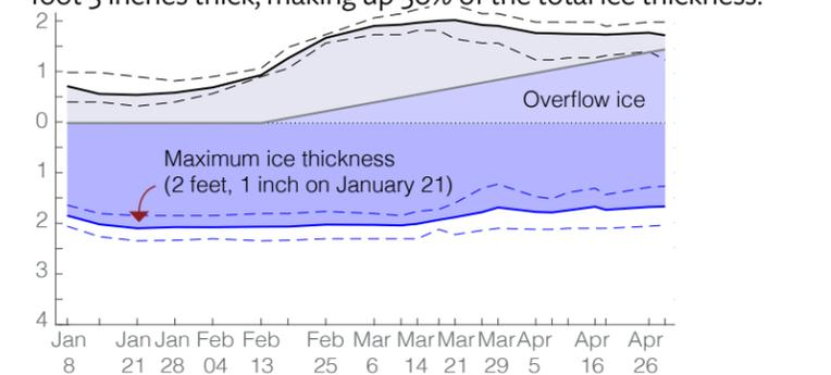
Three consistent patterns emerged. Bay site ice was thicker than in the channel where the current was stronger. Strong winds and thin ice in 2019 caused more flooding so thick overflow ice formed. Ice stopped growing earlier in the winter than expected (ice typically continues growing until mid to late April), which suggests that heat from the ocean limits ice growth.
