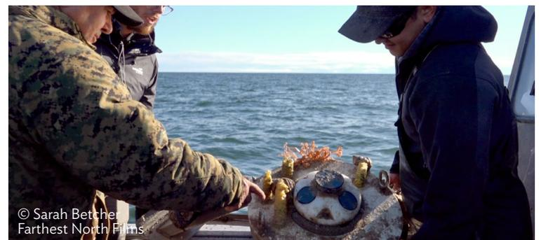
**Ocean mooring** Ikaagvik Sikukun tethered a mooring (science instrument attached to a buoy) in the Sound to measure water temperature.
